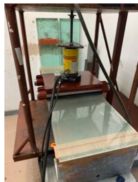
Bending stress test for glass
