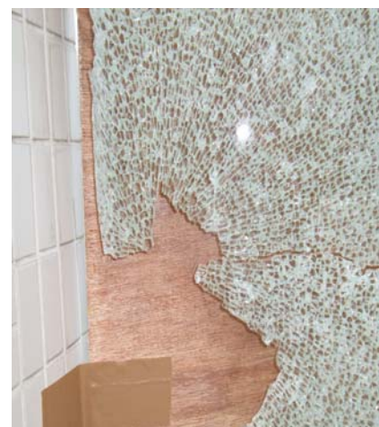
Tempered glass with spontaneous breakage
